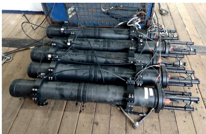
The underwater recorders are deployed to a depth of 1500 m. For species producing low frequency sounds, such as antarctic blue whales, the reception range can be up to 100 km. For high frequency species and seals the range is in tens of km.
